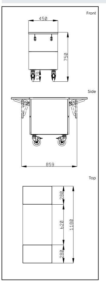
Flexy Compact Ambient unit on cupboard (IGN) with wheels, H=750mm
